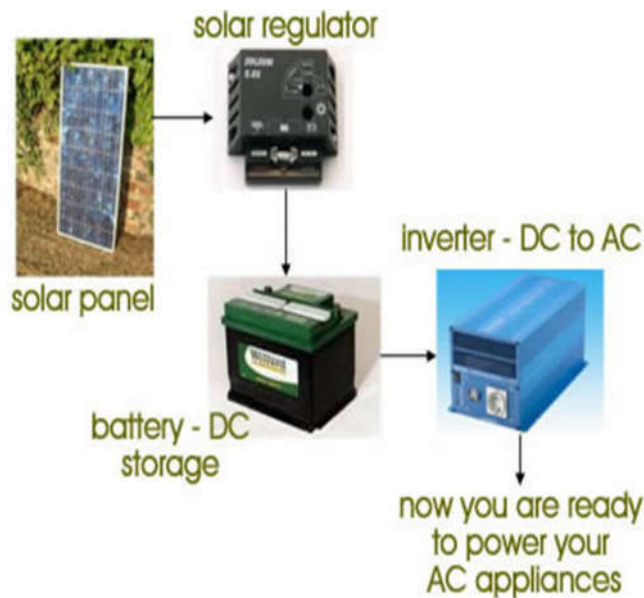
Figure 3 Components of Solar Power System
