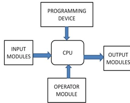
**Figure 2. Block diagram of PLC**
