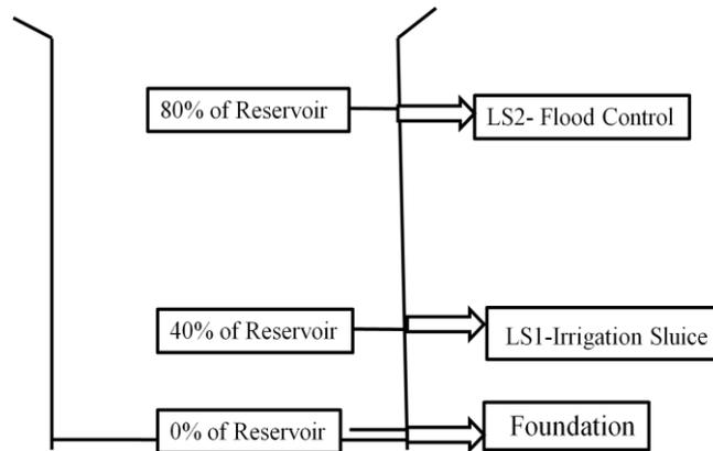
**Figure 3. Layout of Water Reservoir**
