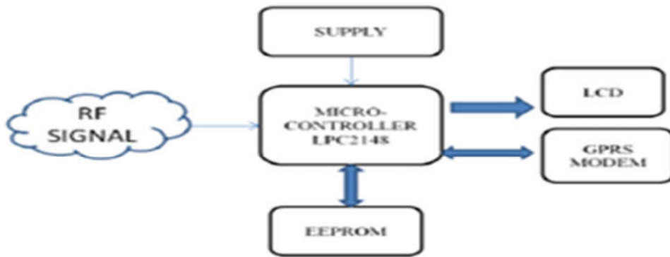
Figure 2: Central controlling unit (Gateway)
