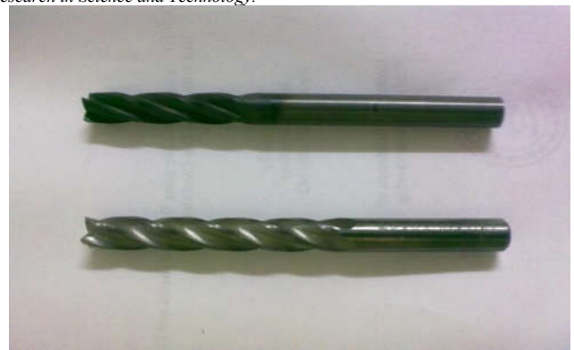
Fig.3 Diamond coated (top) and uncoated (bottom) Tungsten Carbide Tools
