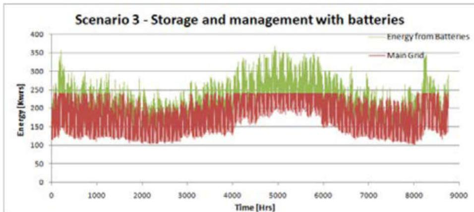
Fig.7 The Energy Demand with Batteries.
