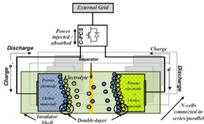
Fig.2 The capacitor storage system [10].
