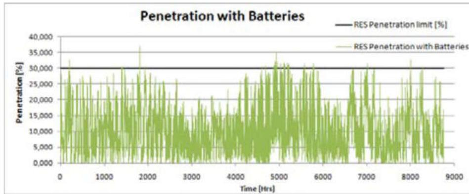
Fig.10 The RES Penetration with the Batteries.
