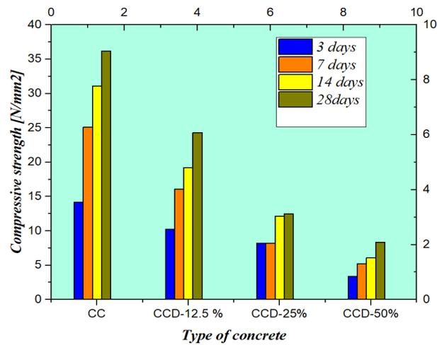
**Figure 1** Types of concrete Vs Compressive strength
