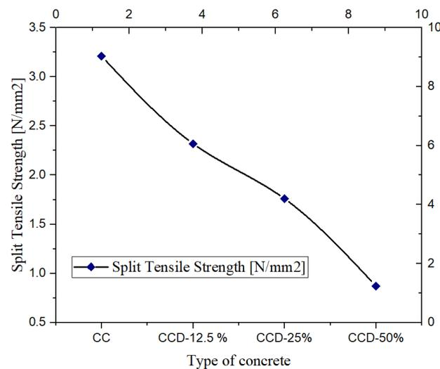
**Figure 2** Types of concrete Vs Split Tensile Strength
