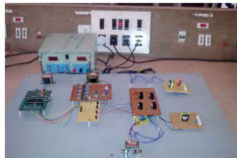
Fig.8. Experimental set up for Bidirectional converter
