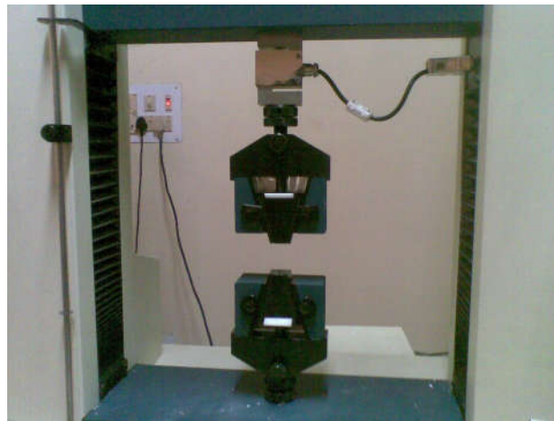
FIG (5.1) UTM machine Sample unloaded condition for tensile testing
