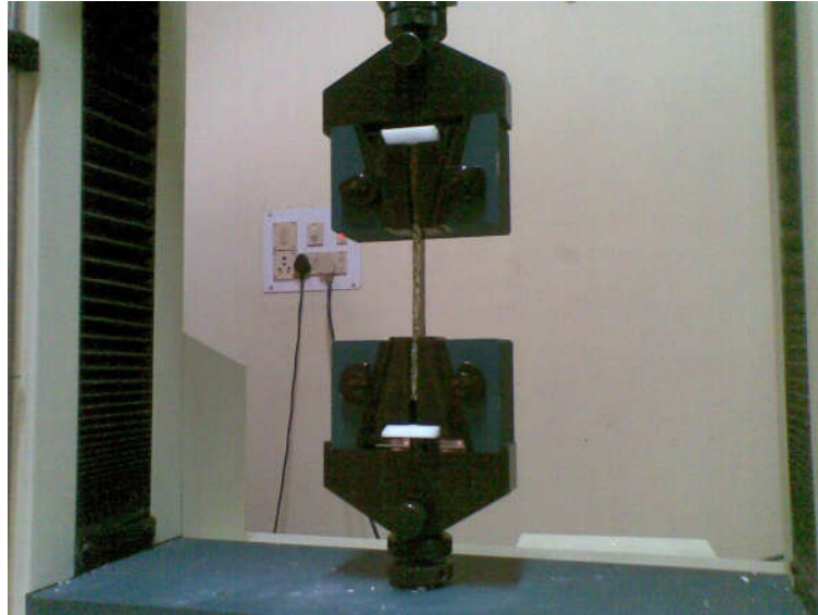
FIG (5.2) UTM machine Sample loaded condition for tensile testing.
